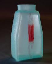
Note the improved adhesion of dyne solution in the treated area.
